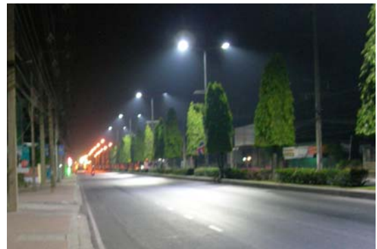
Figure 1 Test site for LED 140W road lighting for M2 class with R3 road surface
